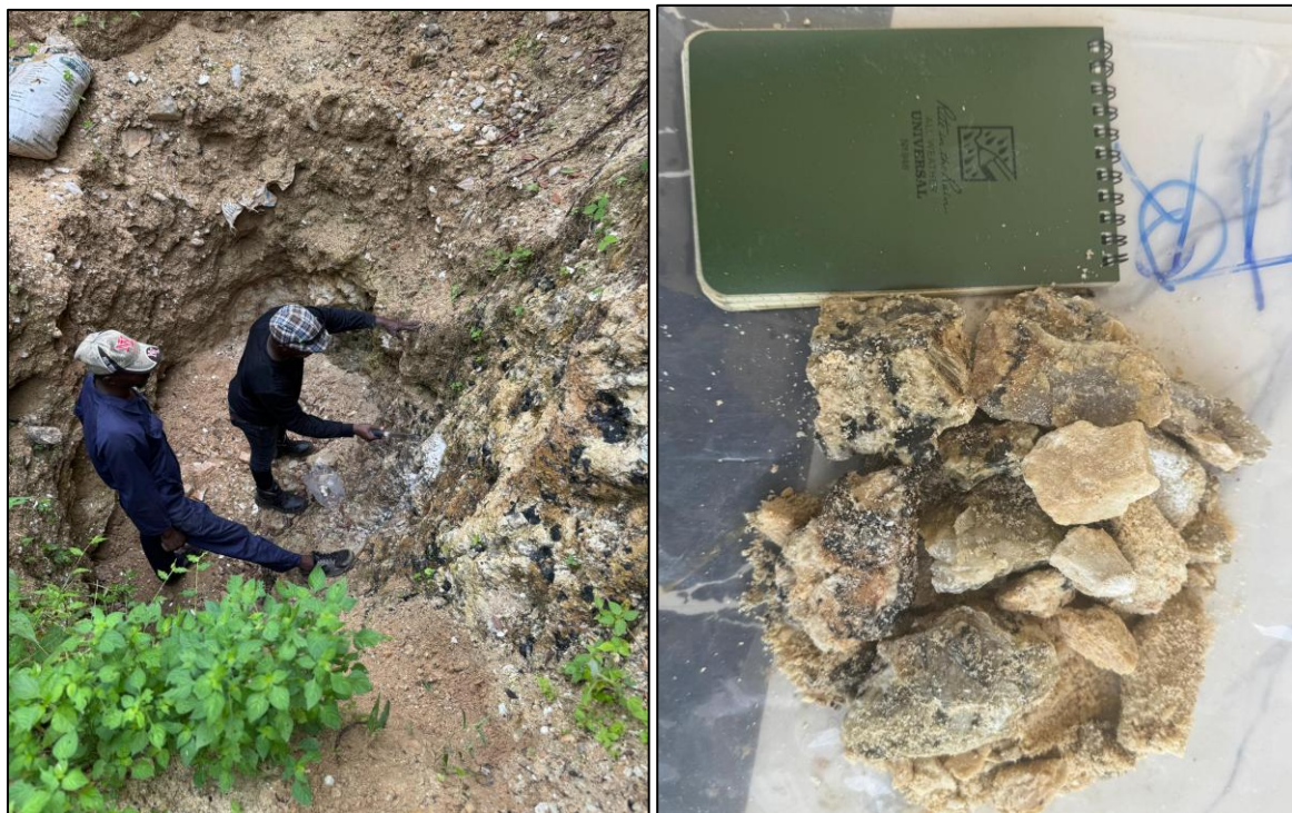
Figure 5: Image showing Geologist collecting a sample in one of the artisanal pits (left) and a sample with spodumene and tantalite mineralisation collected for assaying.
