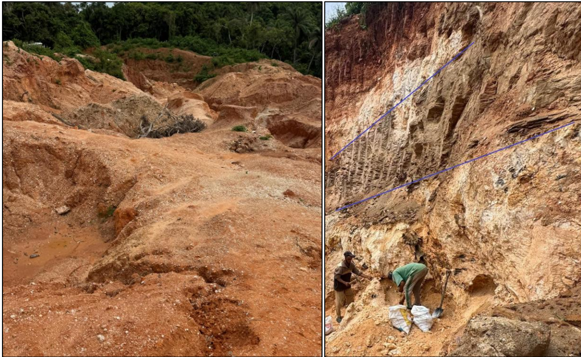
Figure 3: Image showing Ikoro Main pit (left) and pit wall showing the two pegmatite units (in blue line).
