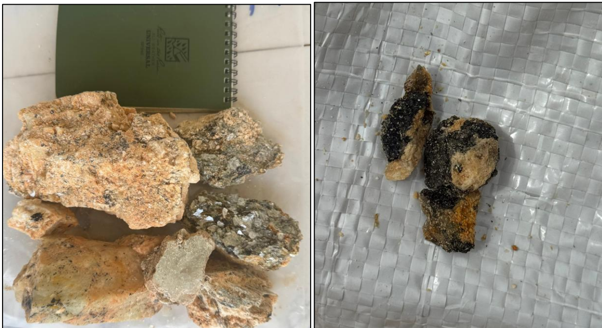
Figure 4: Image of collected sample with spodumene mineralisation (left) and specimen of cassiterite mined at Ikoro main pit (right).
