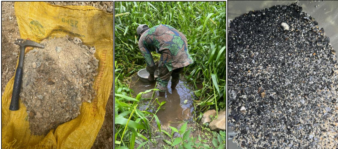
Figure 6: Image showing weathered pegmatite (left), panning of pegmatite (middle) and resulting concentrate made up of tourmaline, tantalite and cassiterite (right).
